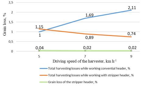
Fig. 4. Grain loss dependence on driving speed
