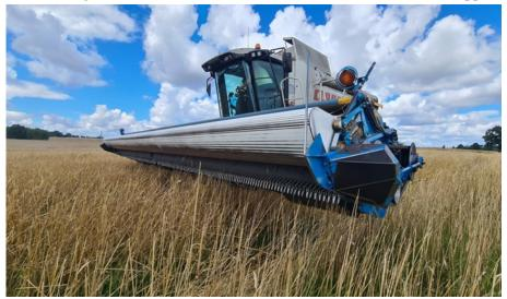
Fig. 1. CLAAS Lexion 550 combine harvester with stripper header
